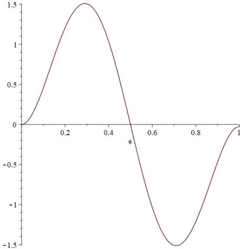
$$Y_3(\varphi) = 0.999386037259572 * (0.999966 \sin(10,9956 \varphi) - \cos(10,9956 \varphi) - 0.999966 \operatorname{sh}(10,9956 \varphi) + \operatorname{ch}(10,9956 \varphi))$$
