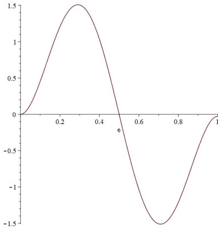
$$Y_3(\varphi) = 0.999966 \sin(10,9956 \varphi) - \cos(10,9956 \varphi) - 0.999966 \operatorname{sh}(10,9956 \varphi) + \operatorname{ch}(10,9956 \varphi)$$
