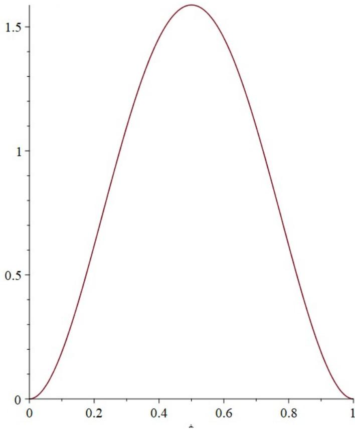
$$Y_2(\varphi) = 0.998118862695376 * (1.0008 \sin(7,8532 \varphi) - \cos(7,8532 \varphi) - 1.0008 \operatorname{sh}(7,8532 \varphi) + \operatorname{ch}(7,8532 \varphi))$$
